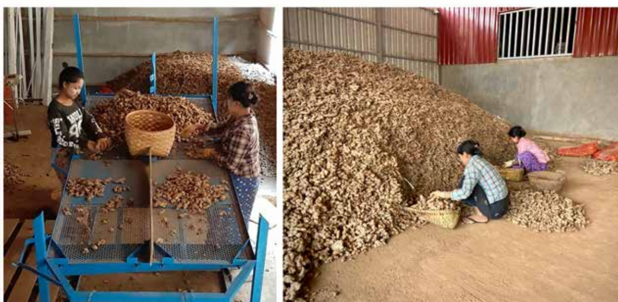
► Image 2 - OSH Adapted Sorting Table (left) vs. Traditional Sorting (right)
