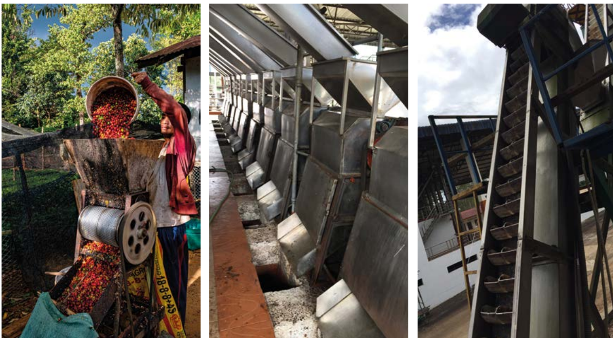
Figure 15. A small-scale “depulping” machine and an industrial-scale pulping facility
